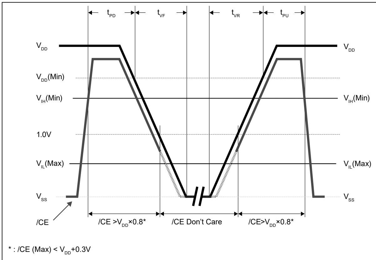
When applying relatively short term VDD pulse whose peak is more than 1.7V, it is required to set falling time,  $t_{VF}$  more than 0.4ms/V. (In case VDD rises over 1.7V and falls just after that, if this term is short, device may lose its function.)
