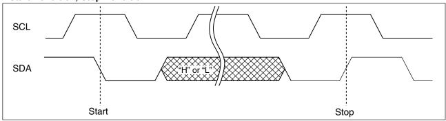
Note: At the write operation, the FeRAM device does not need the programming wait time (twc) after issuing the Stop Condition.
